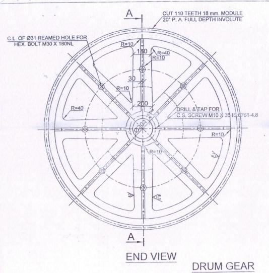
PART NO. - 07-17-02-00-03-01 MATERIAL - GR.3 C.S. 840 OF IS: 2644 - 1994 NOS. PER SET = 02 (TWO) TOTAL NOS. OF SET = 041 FOUR)
